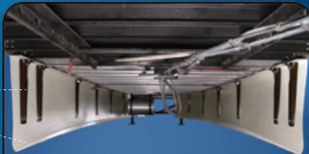
The GREEN WING® trailer skirt features our **exclusive heavy-duty hem**, which improves impact protection and reduces the fairing's weight by more than 10%.
